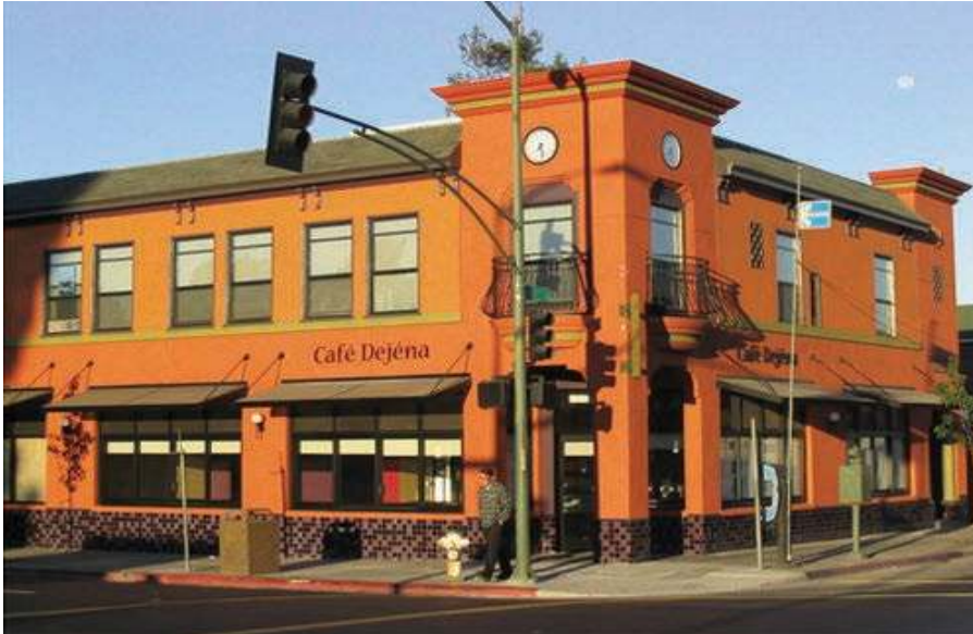
Guideline 7.1.1: The tower feature and corner entrance of this building emphasize the corner location.
